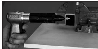
1/4 turn the fastener onto the ARO tool mandrel and place the fastener into the hole.
