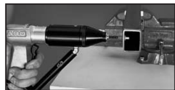
Depress the tool reverse trigger and the tool spins out of the installed fastener.
