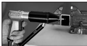
Depress the tool trigger and the tool spins into the fastener and automatically exerts a pressure controlled pull installing the fastener.
