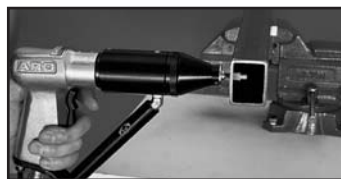
1/4 turn the fastener onto the SPP tool mandrel and place the fastener into the hole.
