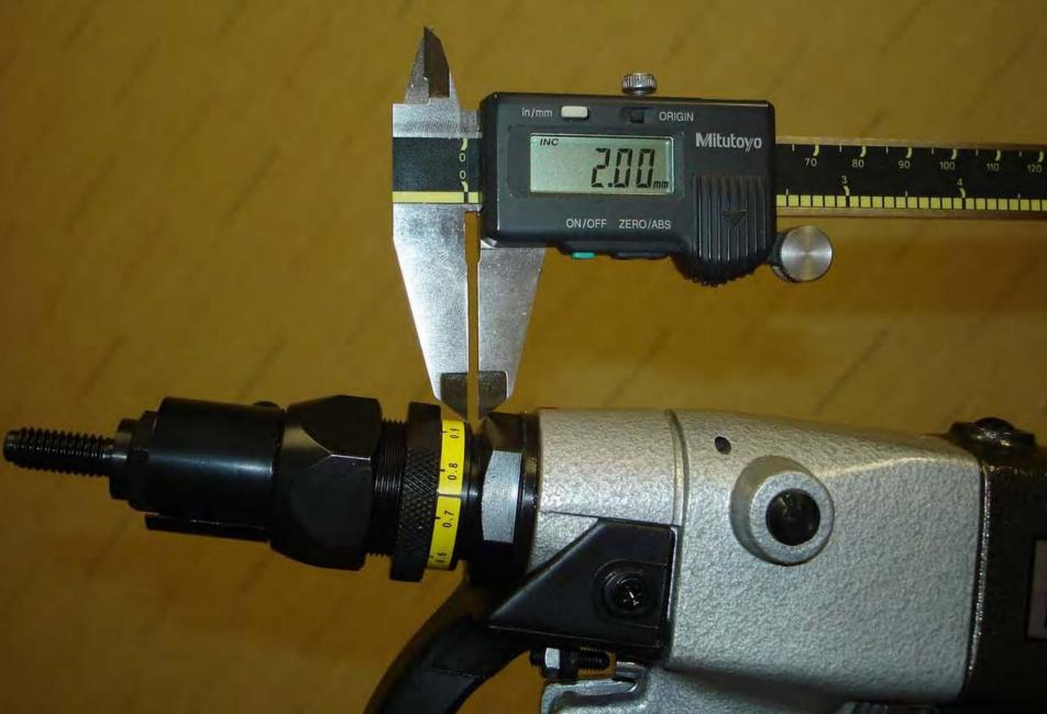
Here the stroke has been adjusted to 5mm. Each revolution of the stroke set nut is equal to 1 mm of stroke. 5 revolutions = 5 mm.
