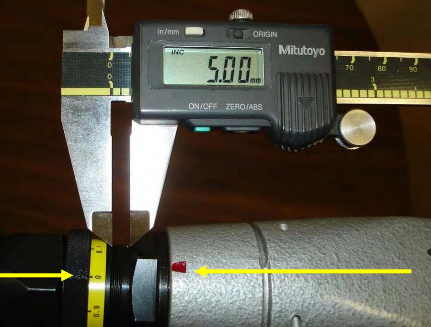
If the rivet nut is not set completely, adjust the stroke out (+1mm); if you experience mandrel breakage, adjust the stroke in (-1mm) until you reach the proper crimp of the rivet nut.
