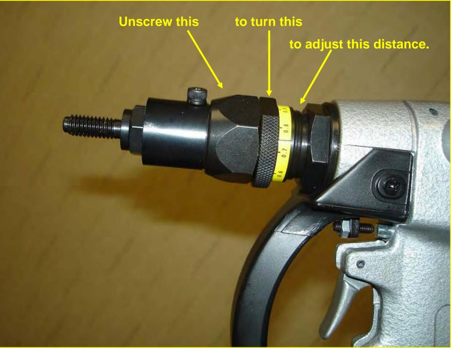
This is the tool with the stroke set at -0-. There is no gap in between the front flange and the base of the stroke set nut.
